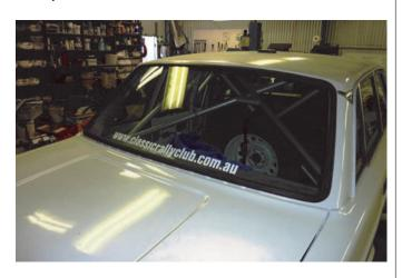
front screen and installed it, the rear screen and the rear quarters – all of which had been removed to fit the cage and paint it. It's starting to look like a car. We should be road testing it at the weekend!!
