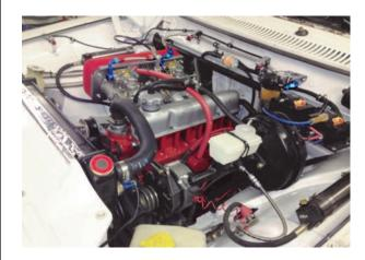
So now the car has an engine and gearbox but not much else. I'd bought new webers in the US, so took them to Tim Howarth at Carburettor Services to check them out and fit them on the manifold with linkages. Tim suggested (very strongly) that the Volvo method of actuating the carbs by means of assorted rods was inappropriate and we should use a cable instead. Luckily the Volvo 240 uses a cable, so we shortened one of those and fitted it and its pedal.
